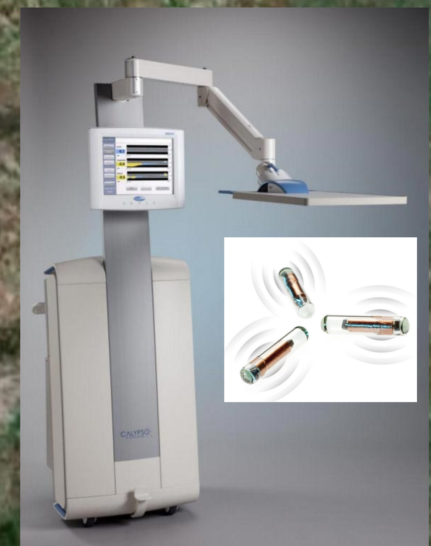
Calypso® System, for real-time tumor motion tracking, developed in Seattle and acquired by Varian in 2011
