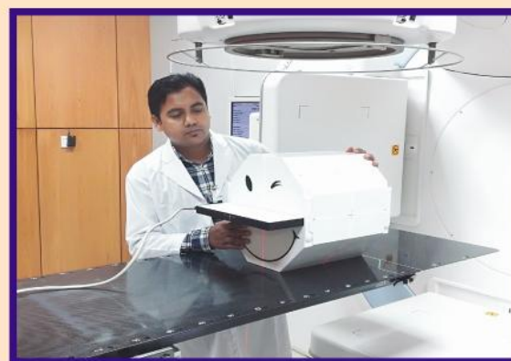
Figure-2: Plan QA using IMRT QA phantom & 2D array
