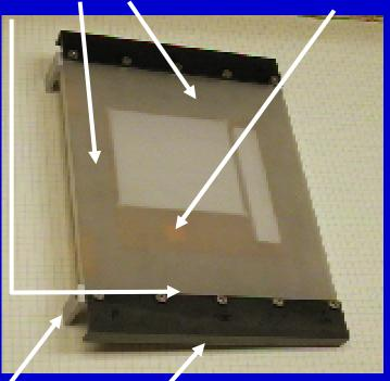
Rulers for measuring distance of detector from chest wall edge of Bucky
