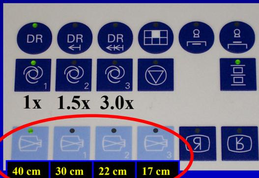
Detector dose scales inversely as either the ratio of the FOV, or as the ratio squared
