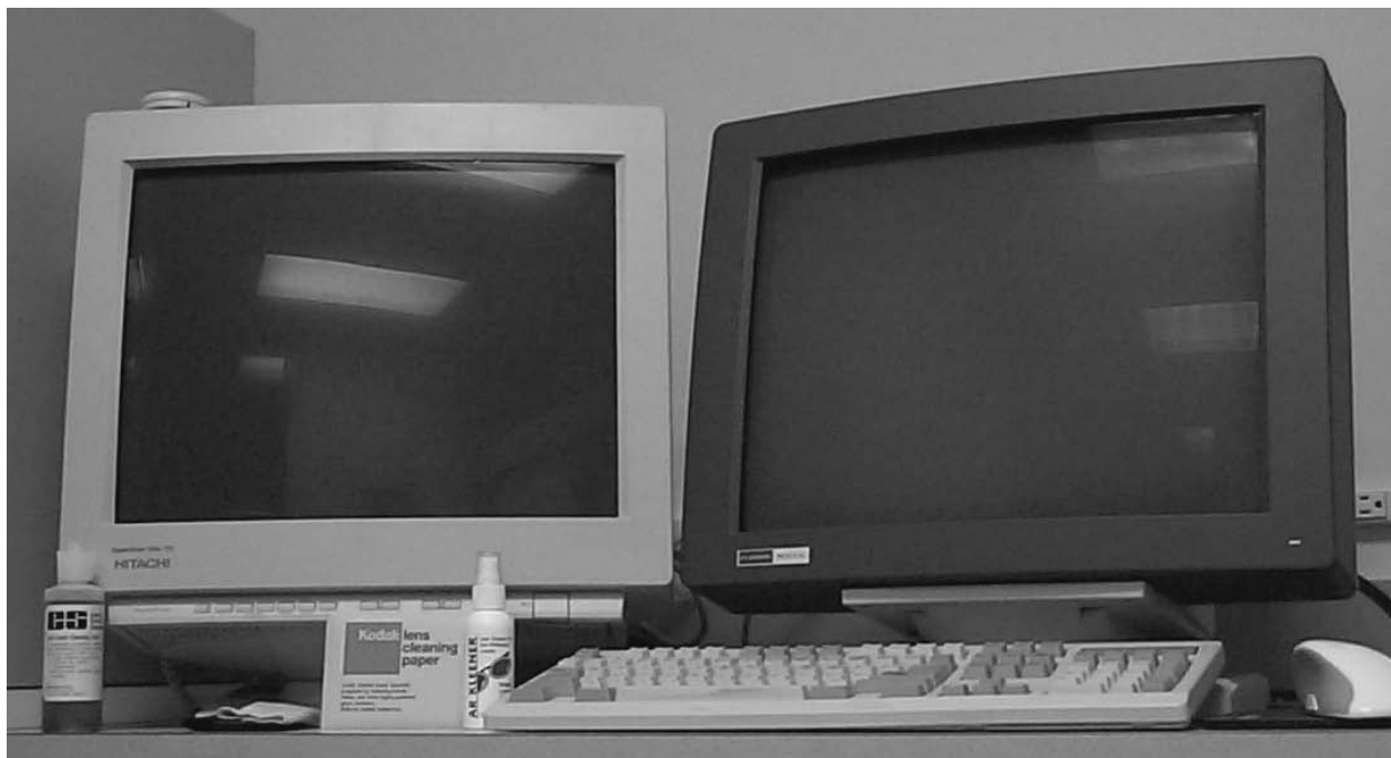
Figure 41. Diffuse and specular reflections are illustrated for a color (left) and a monochrome (right) display device with the power off. Reduced diffuse reflections are seen in the color display device due to the black matrix emissive structure. Reduced specular reflections are seen in the monochrome display device due to an improved anti-reflective coating.
