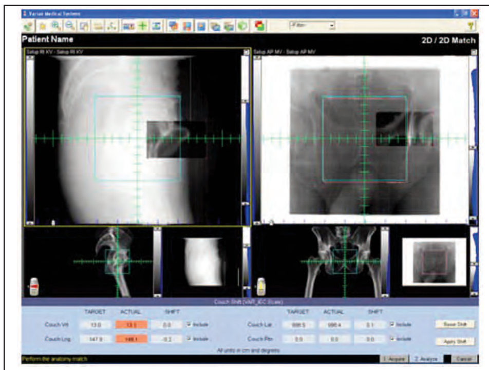
Figure II-C-4. Image analysis tools in the On-Board Imager image-guidance system. Automatic and manual registration methods are available. DRR images, as well as contour projections of the CTV, PTV, or organs at risk, can be overlaid onto the daily images. Translation only or translation and rotation adjustments are calculated. (Courtesy of Fang-Fang Yin, Ph.D., Duke University Medical Center, Durham, NC)
