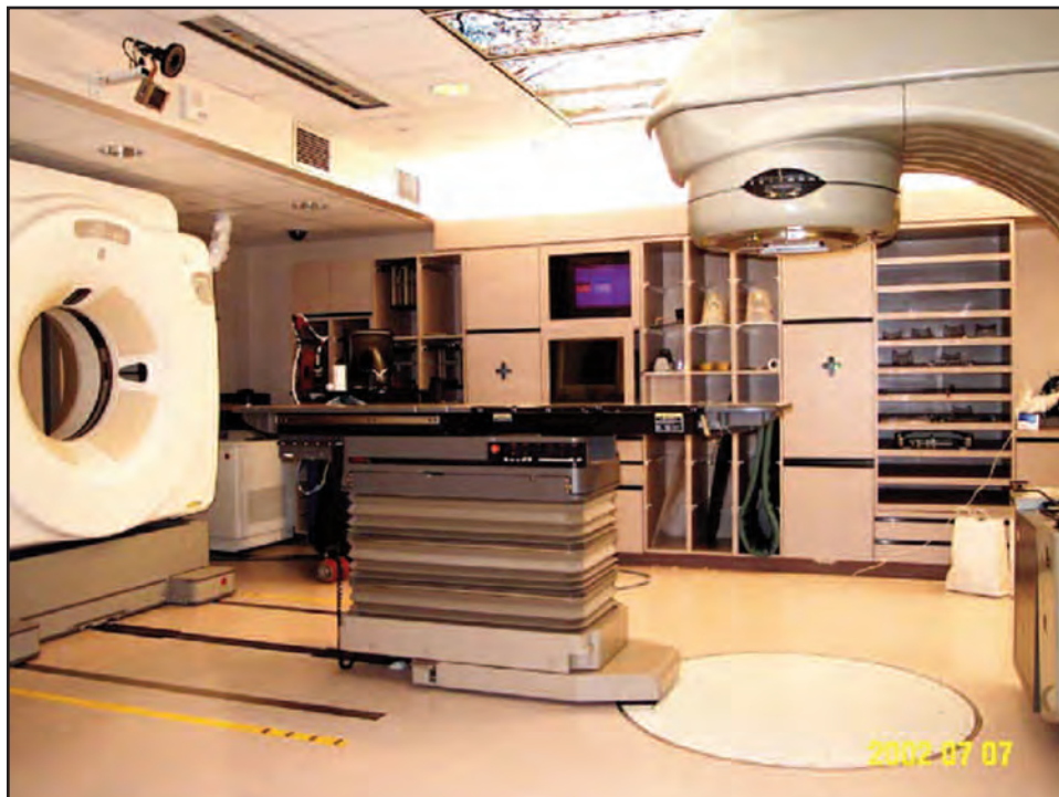
Figure II-A-1. Illustration of a rail-track-mounted system: Varian-GE EXaCT™ system. (Courtesy of Lei Dong, Ph.D., M.D. Anderson Cancer Center, Houston, TX)
