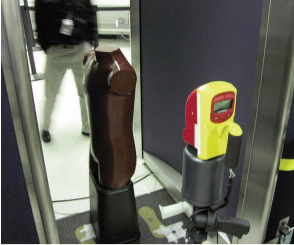
Figure 6. Scatter-leakage measurement setup (Fluke 451p above and Radcal 1800 cc chamber below).
