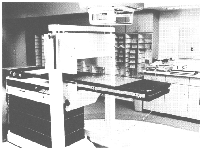
FIG. 10. Photograph of mobile shield positioned over treatment couch.
