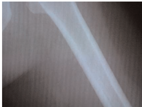
Figure 20. A stationary antiscatter grid can cause aliasing, where the high-frequency patterns are reflected back into the low-frequency spectrum about the Nyquist frequency as superimposed beat patterns.
