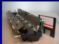
Line-scan CR array reader with "structured" phosphor
