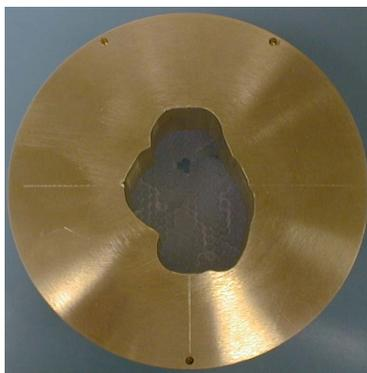
Figure 10: View of a typical brass aperture used to collimate a proton beam. (Bussiere and Adams, 2003)
