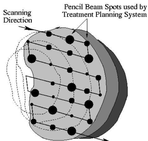
Figure 12: The principle of beam scanning: A narrow pencil beam is scanned across the target volume at various depths. The intensity can be varied from spot to spot, or continuously along the path. (Trofimov and Bortfeld, 2003)
