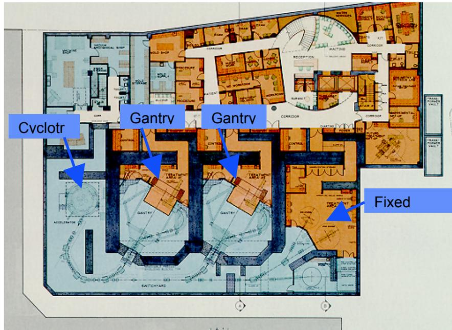
Figure 6: Floor plan of the Northeast Proton Therapy Center. Drawing provided by Ion Beam Applications, S.A.
