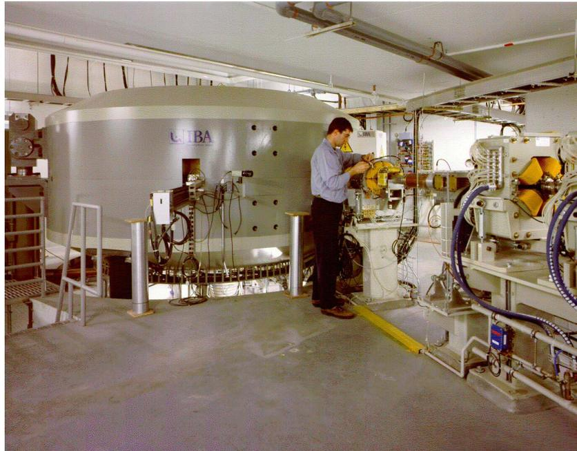
Figure 4 Isochronous cyclotron by Ion beam Applications, S.A. It extracts protons with an energy of 230 MeV, which corresponds to a range of a  $\sim 33.0$  cm in Water. Picture provided by Ion Beam Applications, S.A.
