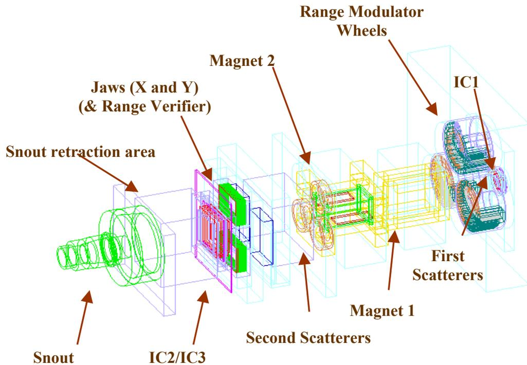
Figure 8: Schematic drawing of the nozzle at the NPTC (Paganetti et al., 2004). Beam monitoring devices are ionization chambers (IC) and a range verifier (multi-layer Faraday cup). Beam shaping devices are scattering systems, range modulators, and wobbling magnets. Variable collimators ('jaws') and the snout determine the field size.
