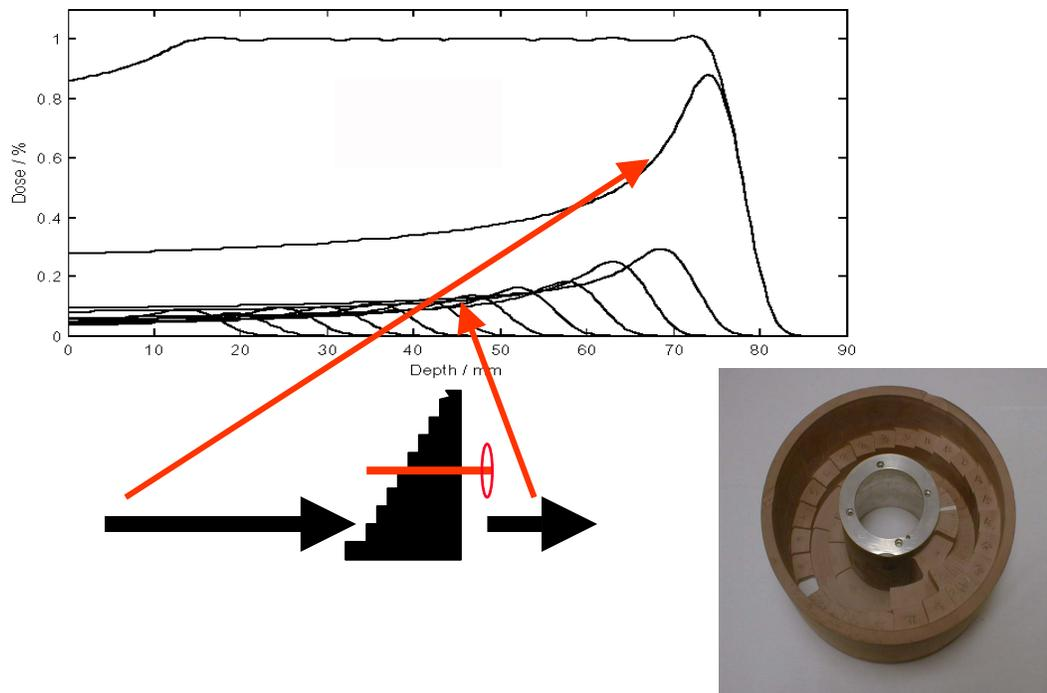
Figure 9 SOBP as composed out of a number of pristine Bragg curves modulated in depth by a set of absorbers of different thickness. The lower right picture shows a wheel with 3 different tracks used for different modulation widths.
