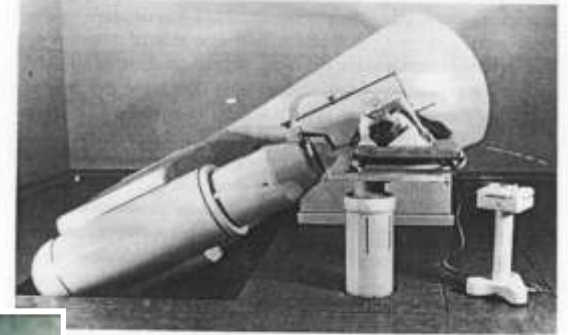
FIG 1-7 · First orientable linear accelerator—The orthotron (from [unclear]).
