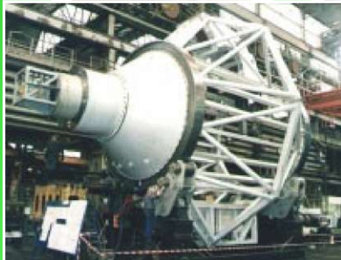
FIG 1-7 · First orientable linear accelerator—The orthotron (from [unclear]).
