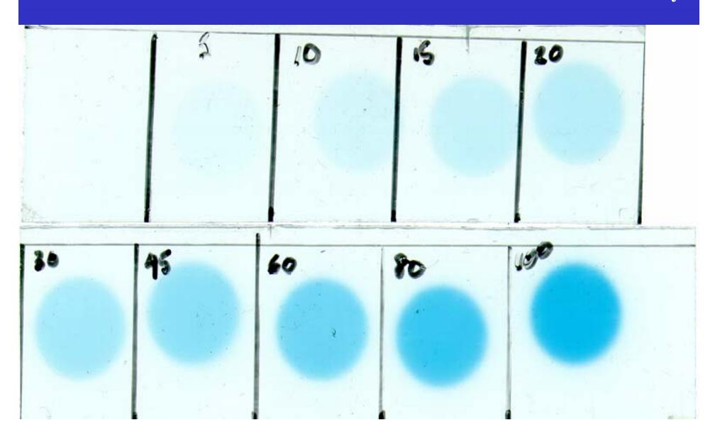
EBT2 Calibration Exposures w/ 60Co in Water
