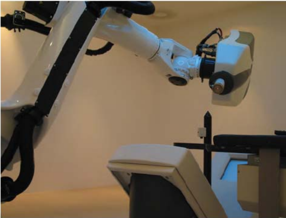
FIG. 3. The black isopost is mechanically mounted on the base frame of the imager system. The isocrystal at the tip of the post defines the coordinate system reference of the CyberKnife ® system. The robot is going through the path calibration process (Sec. III B 1), with the beam laser scanning the isocrystal.
