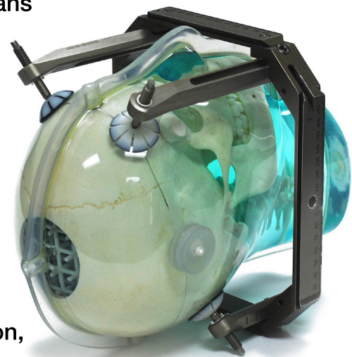
Inter-cranial Grid Phantom 335 Physical Control Points
