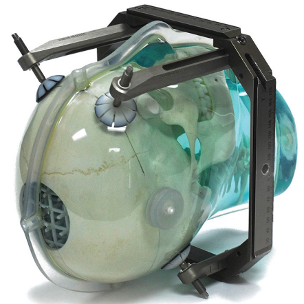
Inter-cranial Grid Phantom 335 Physical Control Points
