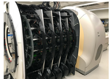
United Imaging's total-body PET scanner at the University of California, Davis. (Courtesy: Ramsey Badawi, PhD, UC Davis)
