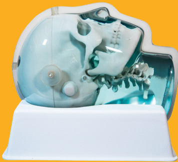
MR Distortion & Image Fusion Head Phantom (603GS)
