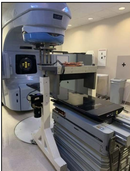
Shielding setup used for treatment of pregnant patients at MD Anderson Cancer Center. Image courtesy of Dr. Sara Thrower.
