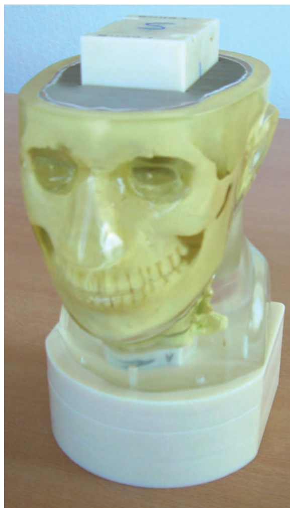
FIG. 5. An anthropomorphic target phantom with the top removed to show the placement of the E2E ballcube to verify tracking accuracy. The top of the smaller ballcube used for Xspine tracking verification can be seen at the base of the cervical spine, labeled with an inverted "A". This phantom shown here can be used to verify cranial, fiducial and Xsight ® Spine tracking.
