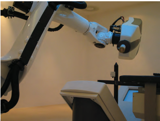
Fig. 3. The black isopost is mechanically mounted on the base frame of the imager system. The isocrystal at the tip of the post defines the coordinate system reference of the CyberKnife ® system. The robot is going through the path calibration process (Sec. III B 1), with the beam laser scanning the isocrystal.
