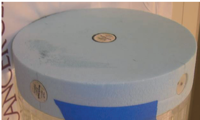
Figure C.2 ^{57}\text{Co} button sources attached to a cylindrical foam block.
