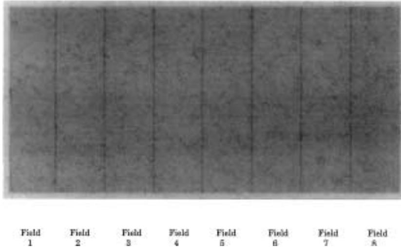
**Figure 11.** Diagram showing the alignment of 5-cm wide strips formed by the MLCs irradiating abutting rectangular fields. The degree of dose uniformity along the match lines is a sensitive measure of the alignment of the leaf position indicators, the light field, and the radiation field.
