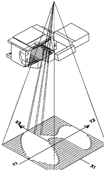
**Figure 4.** Schematic of the General Electric Medical Systems MLC that replaces the lower jaws. The leaves project to a width of 1.25 cm at isocenter so that 32 leaves are used to cover the 40-cm width of the field. A trimmer above the upper jaws is used to refine the penumbra at the leaf ends.
