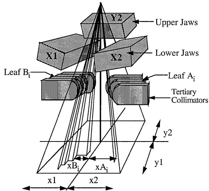
**Figure 2.** Generic schematic of a photon collimation system with upper and lower jaws and a tertiary multileaf collimator. The Y1 jaw has been omitted for clarity. The field dimensions in the plane at isocenter are indicated.
