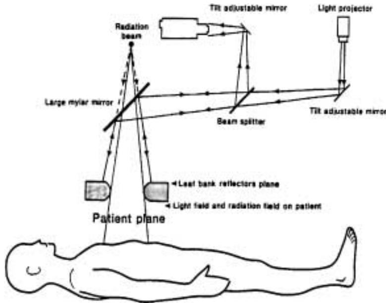
**Figure 9.** Illustration of a video-optical method of determining leaf position.
