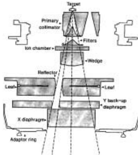
**Figure 3.** Schematic diagram of the Philips MLC. The upper jaw is replaced by the MLC leaves and a back-up diaphragm placed beneath the leaves follows the leaves to provide additional attenuation.
