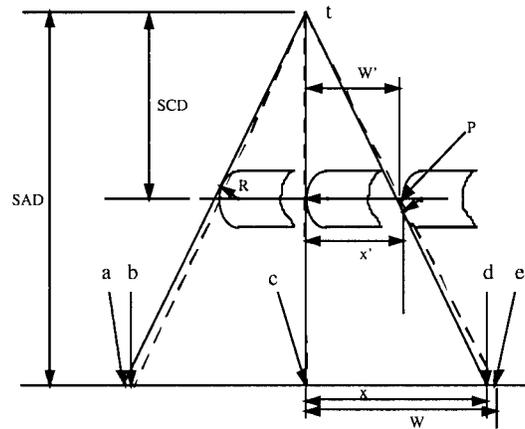
**Figure 8.** Schematic of ray lines that determine the form of the edge of the radiation field and light field at the curved end of an MLC leaf. SAD is the distance from the source to isocenter and SCD is the distance from the source to the center of the leaf. R is the radius of curvature of the leaf end.
