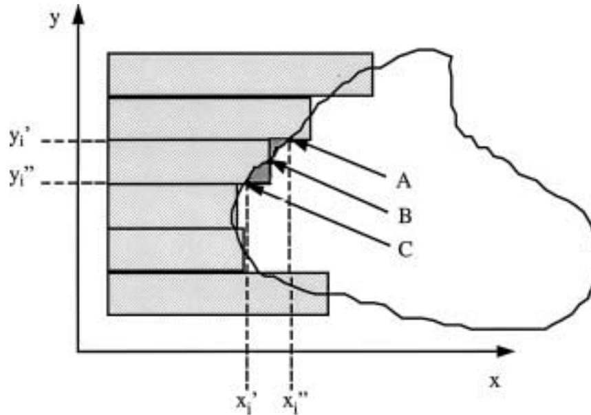
**Figure 13.** Demonstration of the “out-of-field” area between A and B and the “in-field” area between B and C.
