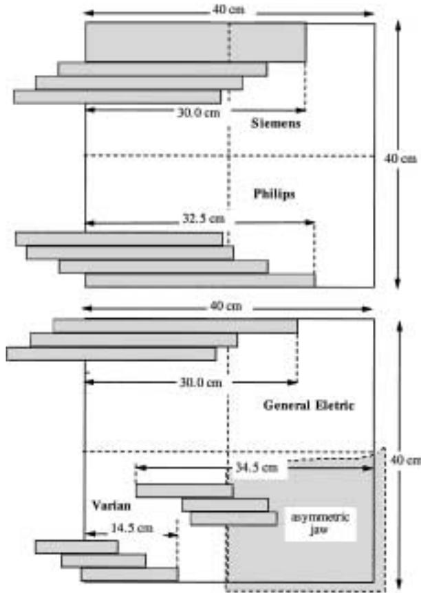
**Figure 5.** A comparison of the leaf travel configurations of commercially available MLCs. The maximum leaf extensions are compared to a 40-cm  $\times$  40-cm maximum field size.
