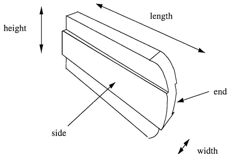
**Figure 1.** Schematic of generic MLC leaf illustrating leaf terminology. An example of a curved end and a stepped side.
