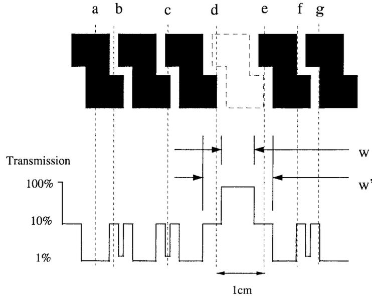
**Figure 7.** Illustration of different leakage paths between leaves and the effect of leaf cross-section shape on penumbra along the side of an MLC leaf.
