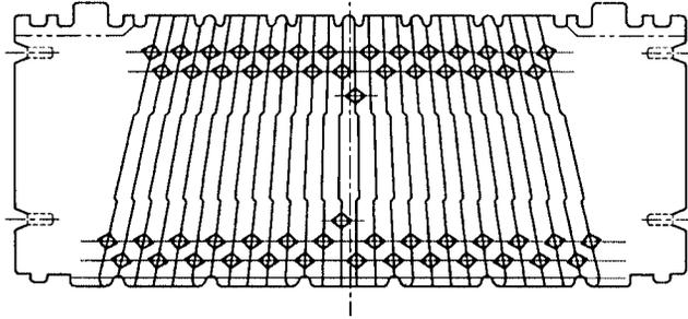
**Figure 6.** End view of the Siemens MLC showing the truncated pie shape of the leaves as well as the leaf side shape to reduce interleaf transmission.
