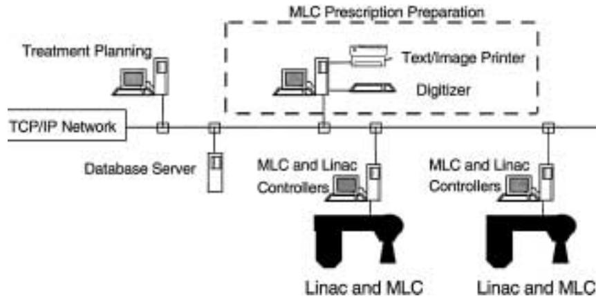
**Figure 10.** Schematic of MLC prescription preparation workstation and its relationship to other parts of the treatment planning and delivery system employing MLCs.
