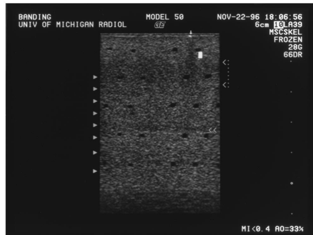
FIG. 2. Examples of common streak nonuniformities. Horizontal bands are often caused by circuitry and focusing problems while vertical bands indicate a damaged transducer element. Drawing (top) and ultrasound image (bottom) illustrating streak nonuniformities. The horizontal streaks in the bottom image are indicated by the open arrowheads that are located on the right-hand side of the phantom.
